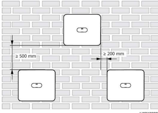
**Figure 4-4** Triangle installation mode (recommended)
