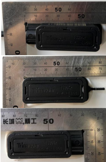
Fig. 15: detail view of closed junction box
