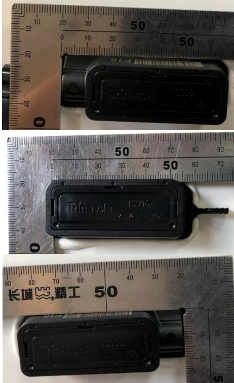
Fig. 5: detail view of closed junction box
